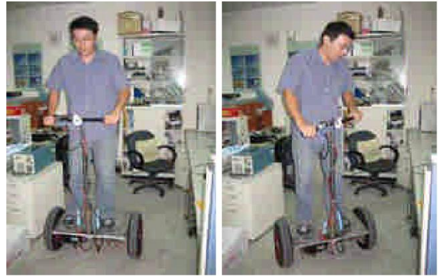
Fig.10 Experimental picture of the human driver's self-balancing control.
